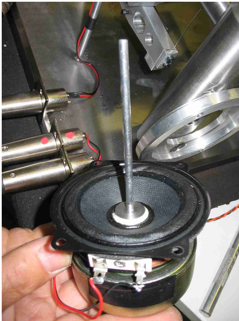
Figure 3 Using loudspeaker as a vibration velocity sensor
