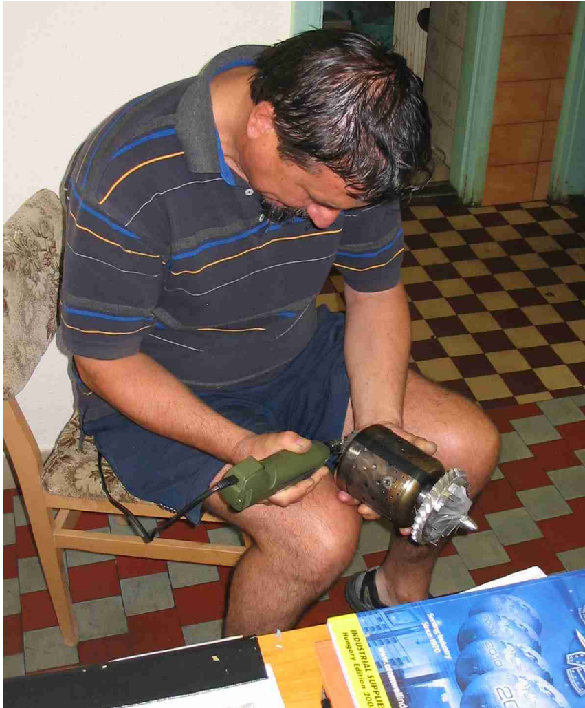
Figure 17 János Horváth is grinding his turbine
