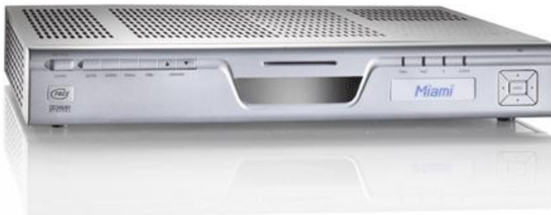
2.8. ábra - Pace Micro Technology Miami DC757 HD Set Top Box
