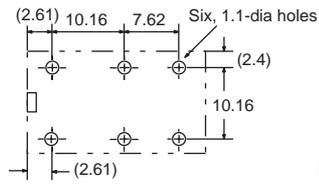
**Mounting Height of Relay with Connecting Socket**
