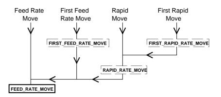
In the diagram a statement within a dashed box is optional, the FEED\_RATE\_MOVE is compulsory and hence is always present. The diagram indicates that for a first rapid move, the post processor first tries to format the output using the FIRST\_RAPID\_MOVE statement. If this statement does not exist the RAPID\_RATE\_MOVE statement is used. If this statement does not exist the FEED\_RATE\_MOVE statement is used. The other types of moves follow a similar route as shown on the diagram.
