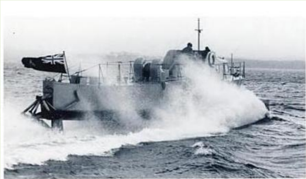
When the first Bras d'Or was launched, she had considerable difficulties in maintaining foilborne stability.
