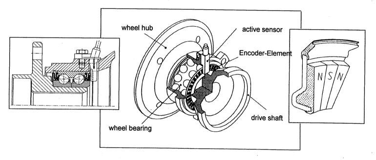
Figure 2: Hub Unit with Active Encoder Seal and Active Sensor
