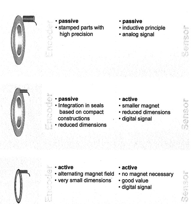
Bigger Air-Gap, Zero-Speed Detection Possibility of High Integration
