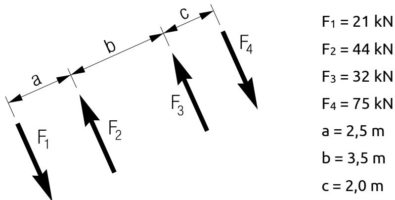
$$R = F_1 + F_2 + F_3 + F_4 = 21 \text{ kN} - 44 \text{ kN} - 32 \text{ kN} + 75 \text{ kN} = \mathbf{20 \text{ kN}} \quad [4 \text{ p}]$$
