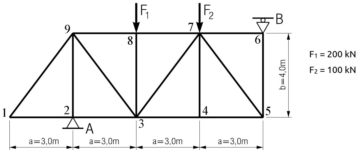
$$\begin{aligned}\Sigma M_A &= 0 = F_1 \cdot a + F_2 \cdot 2 \cdot a + B \cdot 3 \cdot a = 200 \text{ kN} \cdot 3,0 \text{ m} + 100 \text{ kN} \cdot 6,0 \text{ m} + B \cdot 9,0 \text{ m} \\ &= 600 \text{ kNm} + 600 \text{ kNm} + B \cdot 9,0 \text{ m} = 1200 \text{ kNm} + B \cdot 9,0 \text{ m}\end{aligned}$$
