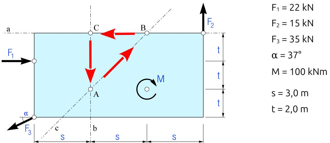
$$F_{3x} = F_3 \cdot \cos \alpha = 35 \text{ kN} \cdot \cos 37^\circ = 27,952 \text{ kN} (\leftarrow) [0,5 \text{ p}]$$
