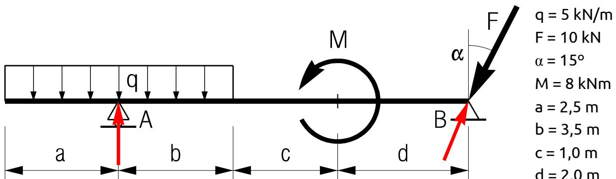
$$F_x = F \cdot \sin \alpha = 10 \text{ kN} \cdot \sin 15^\circ = 2,588 \text{ kN} \quad (\leftarrow) \quad [1 \text{ p}]$$
