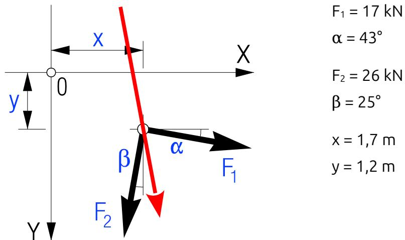
$$F_{1x} = F_1 \cdot \cos \alpha = 17 \text{ kN} \cdot \cos 43^\circ = \mathbf{12,433 \text{ kN}} (\rightarrow) [0,5 \text{ p}]$$
