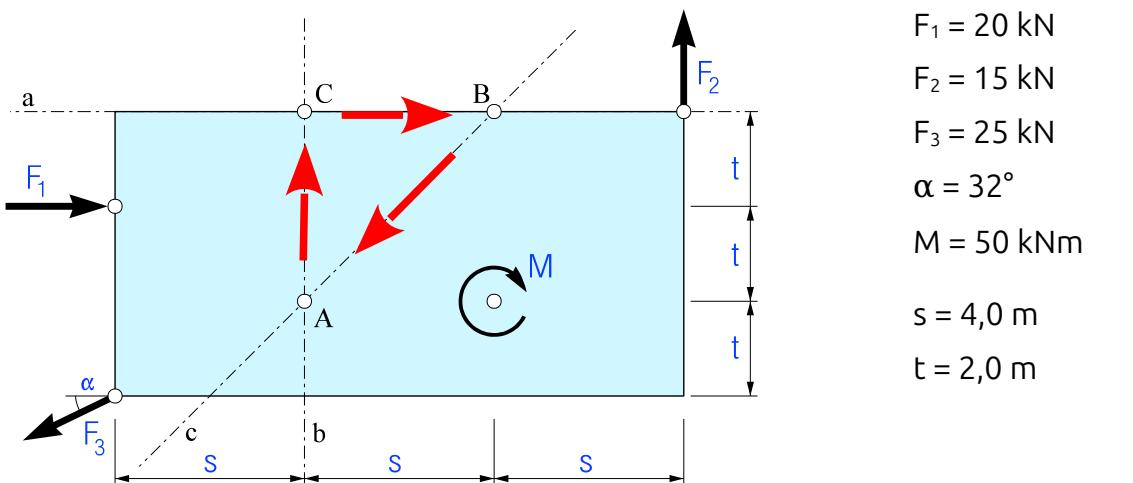
$$F_{3x} = F_3 \cdot \cos \alpha = 25 \text{ kN} \cdot \cos 32^\circ = 21,201 \text{ kN} (\leftarrow) [0,5 \text{ p}]$$
