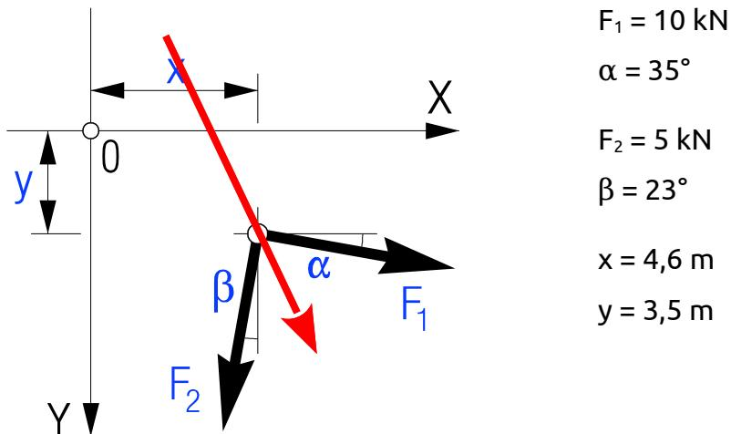
$$F_{1x} = F_1 \cdot \cos \alpha = 10 \text{ kN} \cdot \cos 35^\circ = 8,192 \text{ kN} (\rightarrow) [0,5 \text{ p}]$$
