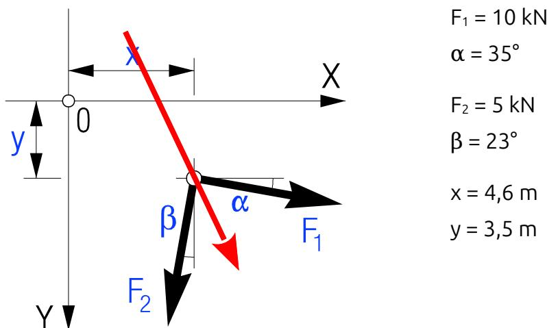
$$F_{1x} = F_1 \cdot \cos \alpha = 10 \text{ kN} \cdot \cos 35^\circ = \mathbf{8,192 \text{ kN}} (\rightarrow) [0,5 \text{ p}]$$
